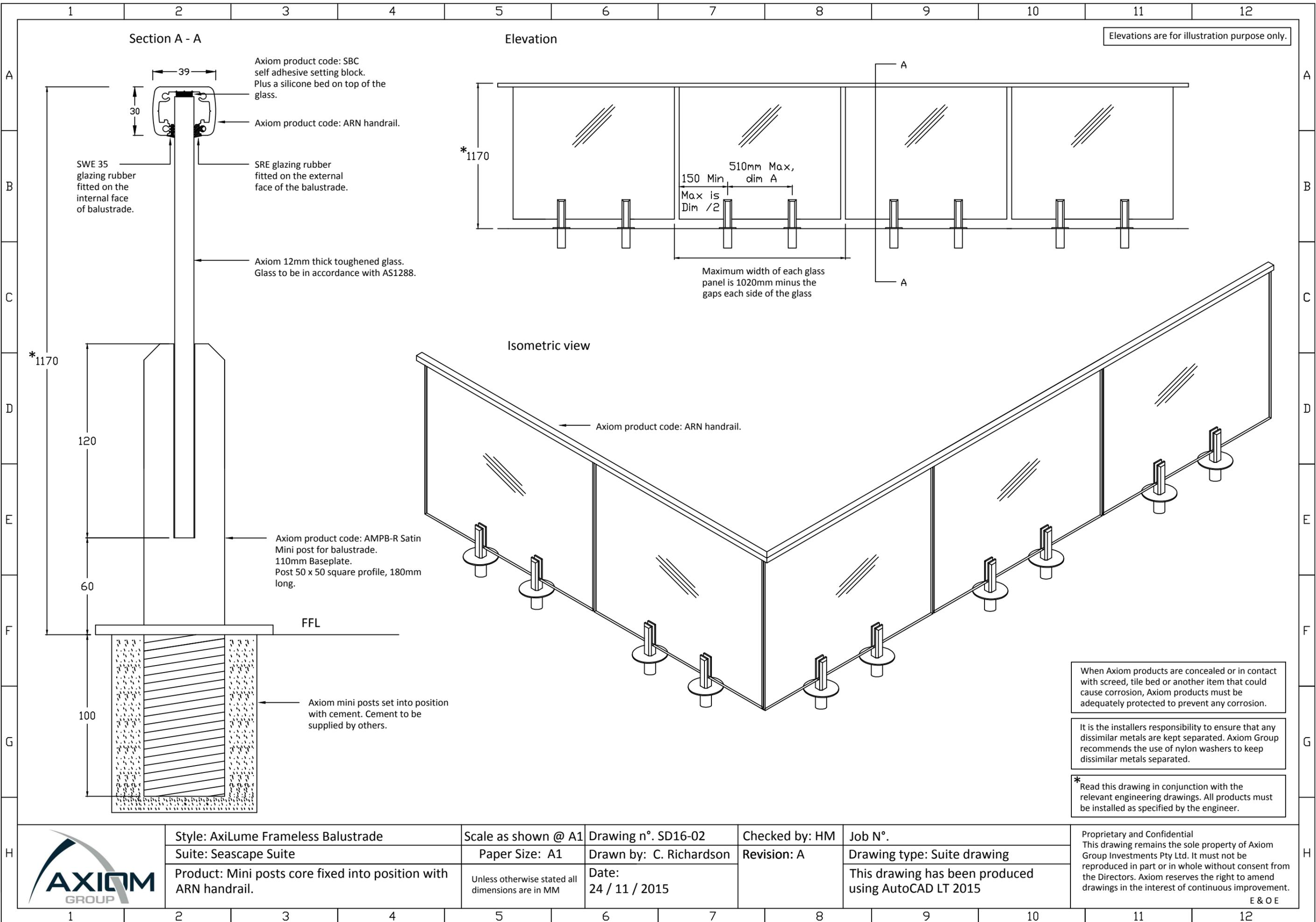
When Axiom products are concealed or in contact with screed, tile bed or another item that could cause corrosion, Axiom products must be adequately protected to prevent any corrosion.
